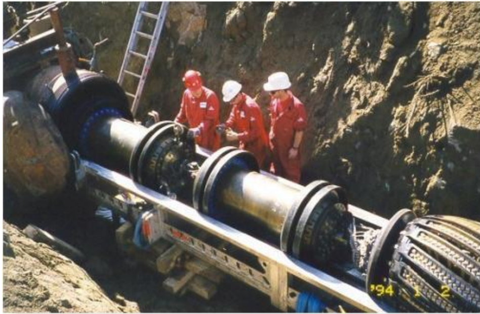
Figure E.2: Shear Wave Ultrasonic Tool Being Launched from a Temporary Launch Barrel.
