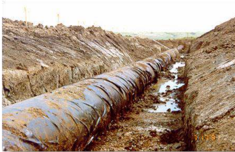
Figure 2.3: Disbonded Polyethylene Tape.
