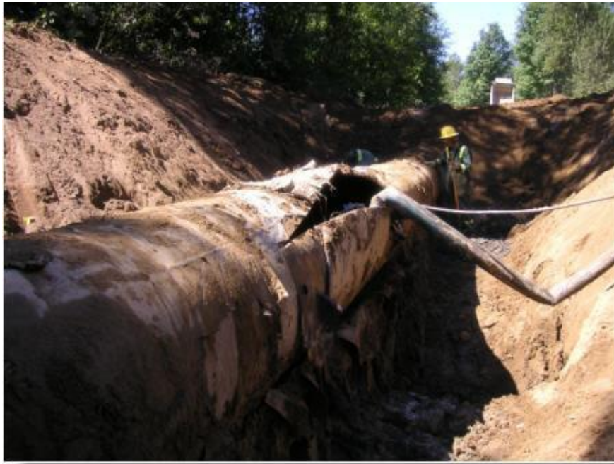
Figure E.9: Excavated Hydrostatic Test Failure.
