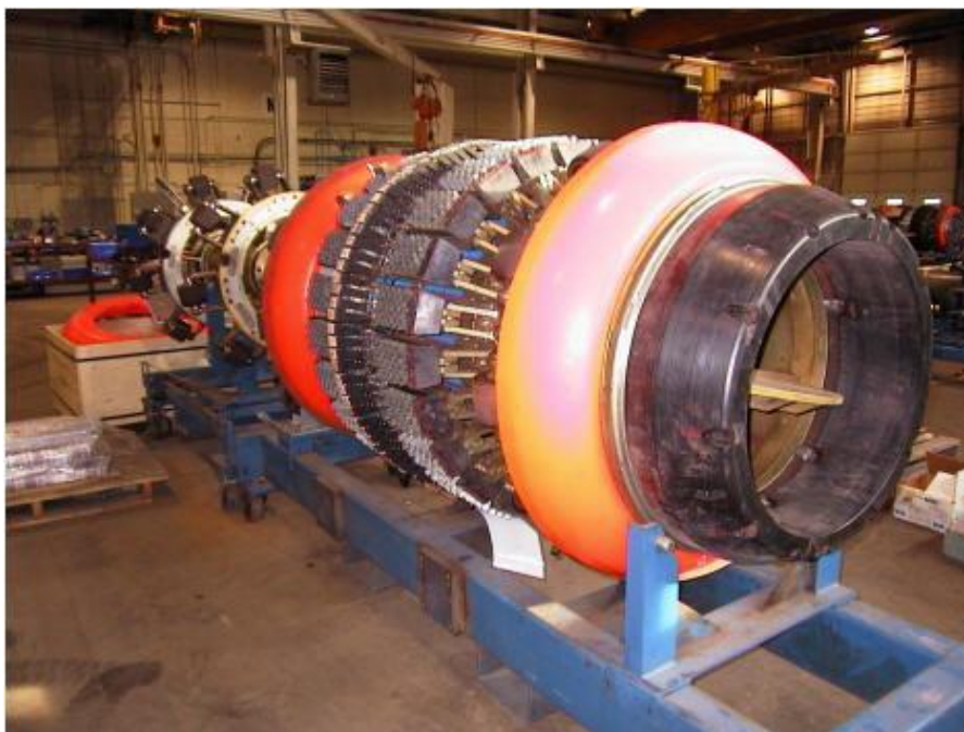
Figure E.1: MFL ILI Tool with Variable Bypass to Allow Product to Flow Through the Internal Bore with Tool Travel Speed Controlled by Valves.
