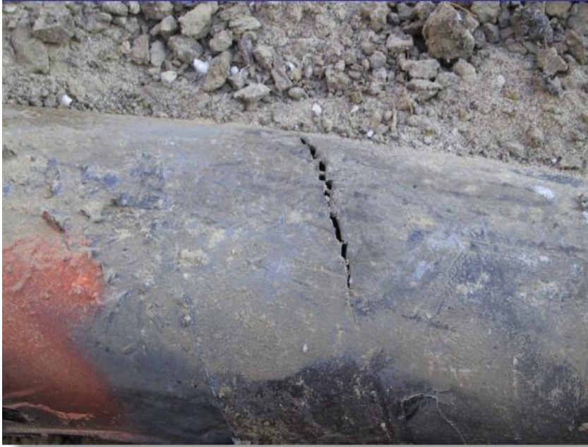
Figure C.4: Circumferentially-oriented Cracks that Resulted in a Leak in an NPS 8 Pipe.
