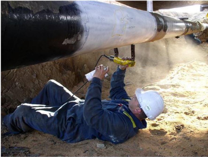
Figure B.1: Bottom of Pipe In-the Ditch SCC Assessment Using BWMPI.
